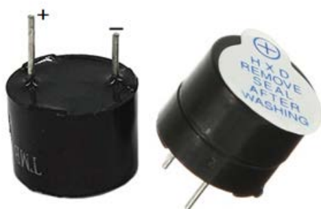
Fig. 8. The buzzer and its pins
